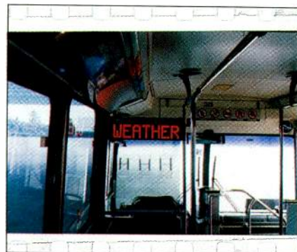
An active LED sign on a Dallas Area Rapid Transit bus, fed by an FM data subcarrier. The 27" x 6" display can produce text and graphics. News, weather, sports, trivia, transit system information and advertisements are carried on the service, which employs a 4.8kbit/s datastream on a 67kHz subcarrier of KJMZ-FM, Dallas, 100.3MHz. (Courtesy of Modulation Sciences.)
