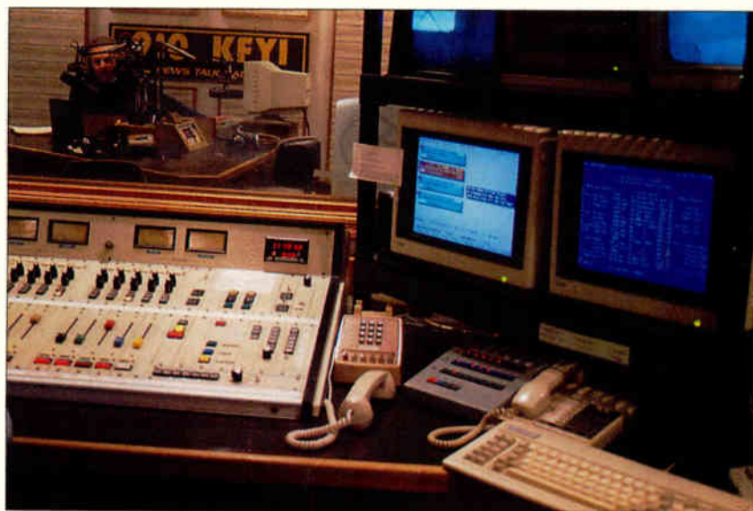
Call screening station in control room at KFYI, Phoenix. Light blue graphics screen (left monitor on lower shelf) shows caller data. This display also appears on host's monitor in studio.
