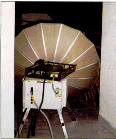
Rear view of MAGNAPhone shows codec (black box) connecting to transmit/receive unit via V.35 cable. The black cable at center feeds audio from mixer to codec. The gray cable snaking off to the right connects the control console to the transceiver.
