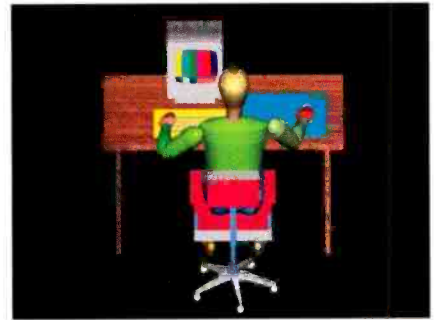
Figure 5. Keyboard and digitizer produces bad shoulder angles (45°) and constant head and neck movement when moving from monitor to keyboard to pad. (Courtesy of VidCAD.)
