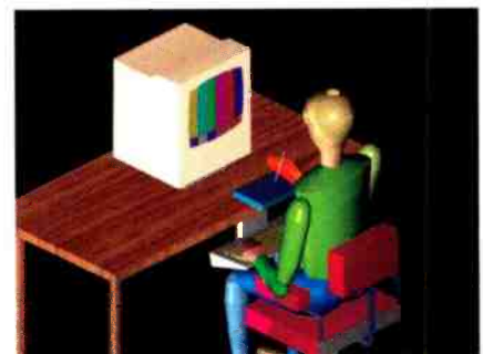
Figure 6. Keyboard on articulated shelf with digitizer on top puts keyboard, small digitizer and monitor in more comfortable position.
