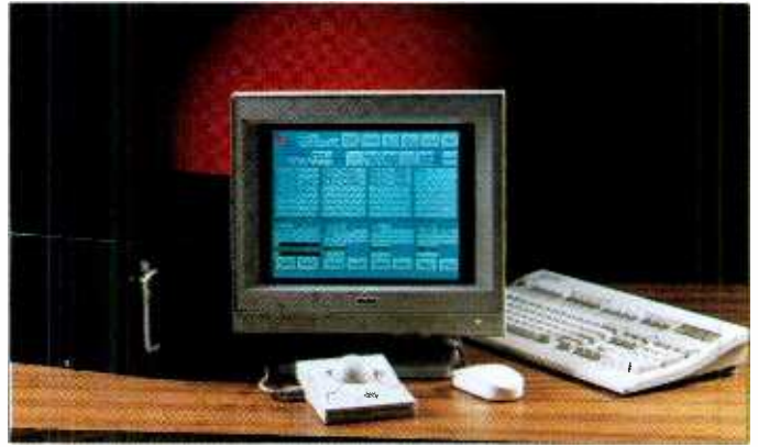
A typical desktop radio system includes a rack-mountable CPU/disk drive, a VGA monitor, a trackball or mouse and a QWERTY keyboard.
