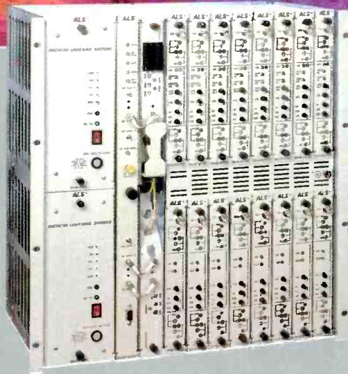
The DV6000, 2.4 Gb/s, sixteen channel system with powerful drop/add/pass capability
