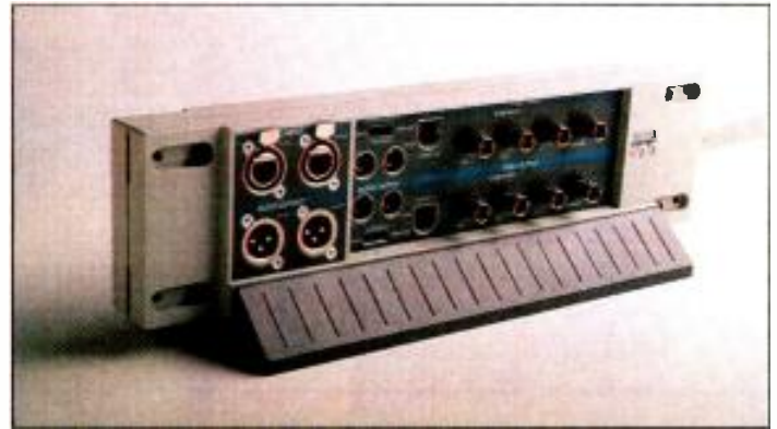
Connector panel used with a desktop non-linear system. Panel can be used on a tabletop or rack-mounted for easy connection. (Photo courtesy of Data Translation.)
