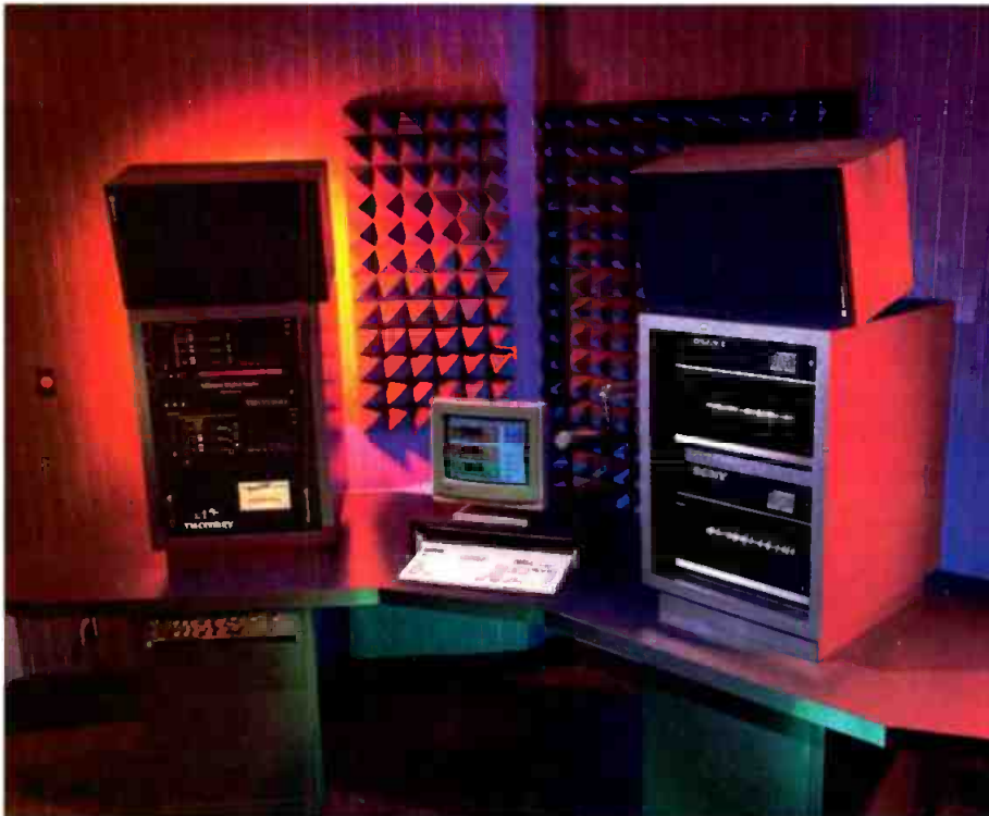
TM Century's Ultimate Digital Studio (UDS) system is another popular audio management platform, shown here with outboard CD jukebox drives (at right).
