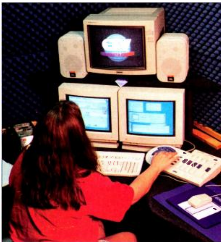
A mid-range non-linear editing system that uses wavelet compression. Because the system is compact, it can be located almost anywhere. (Photo courtesy of Immix.)
