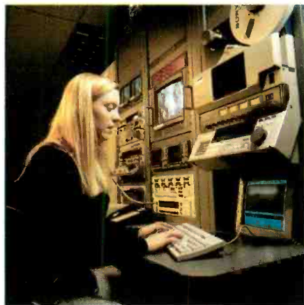
The Turbodisk media management system can be used for dubbing in source material.
