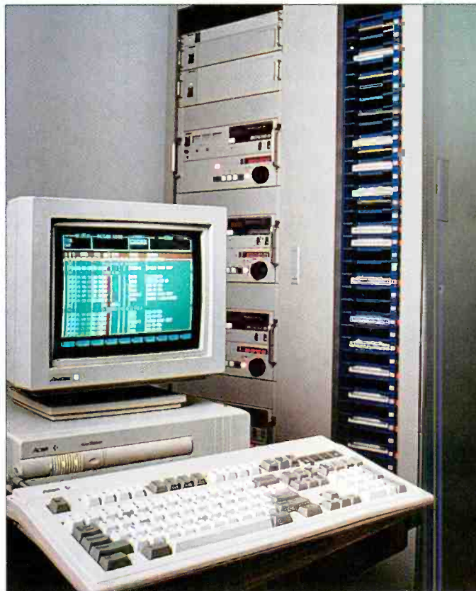
The basic components needed for the TAS automation system include a PC-compatible computer, TAS software and a tape library system.
