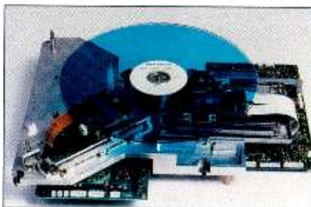
The transport mechanism of the Digital LD is shown above. On this unit, one optical pickup is used for playback and the other is for record. Units can be configured for up to four simultaneous output channels from a single side. A 2-pickup unit can provide outputs from both sides. However, only one pickup at a time can be used because the disk rotation must be reversed.
