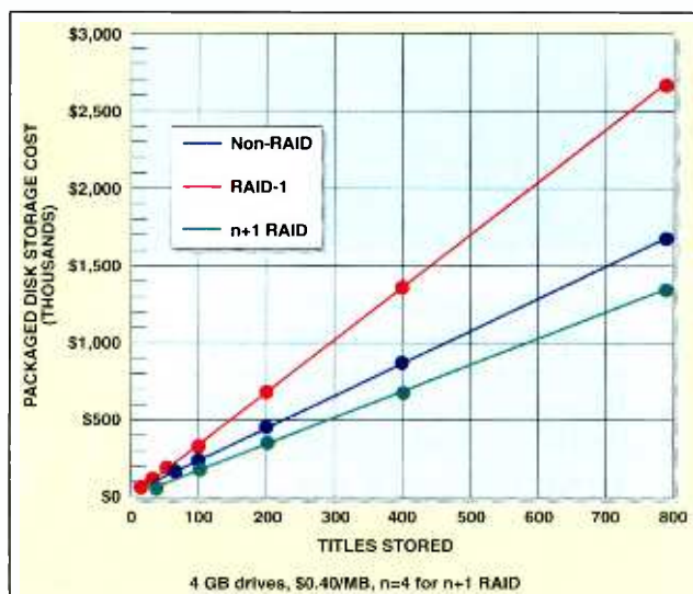
Figure 2. This chart shows the typical storage costs for varying number of compressed (3Mb/s video rate) 2-hour movies. Shown are costs for non-redundant, n+1 RAID and mirroring (RAID-1) configurations.
