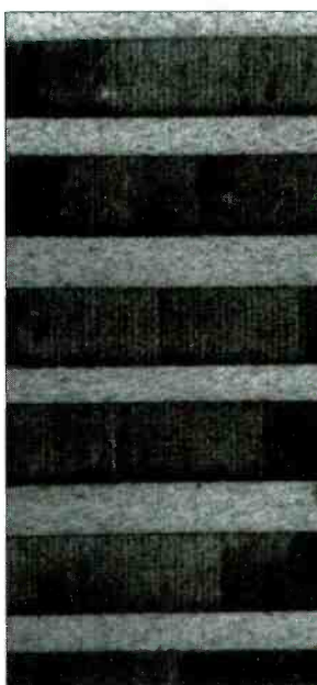
Tracks used for the U-matic format are shown in the diagram. Photo shows the video tracks magnified 100x. The dark area is the recorded information, with the lighter areas used as guard bands. Guard bands are approximately .05mm, the diameter of a human hair.
