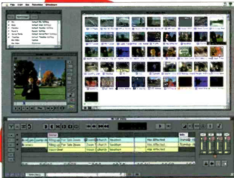
NewsCutter is a server-based editing system that allows multiple users to access and edit the same material simultaneously, each for different applications.
