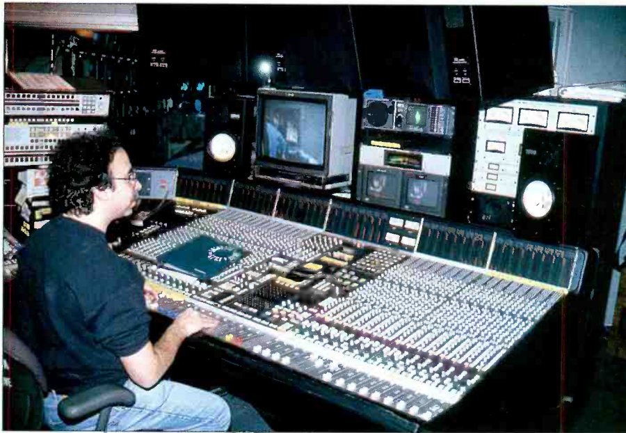
The production control room for NBC's Studio 8H and mixer Bob Palladino handle the live air mix for SNL. Note multiple monitoring systems, including large speakers overhead (L-C-R), stereo pair on console meter bridge and mono mini-speaker next to video monitors.
