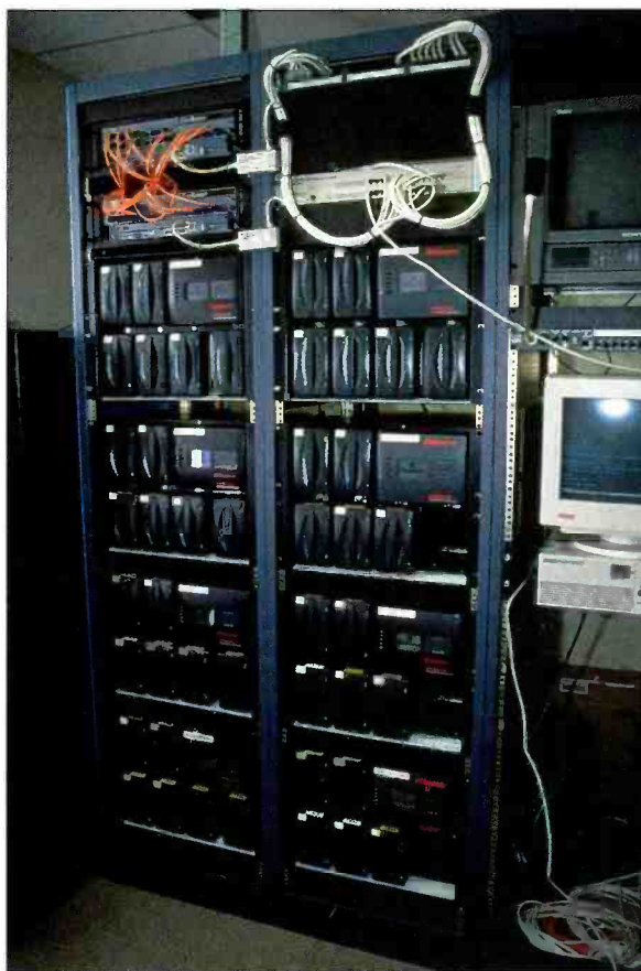
The SGI Challenge Series server and Megadrive storage used by the MediaServer at North West Cable News. It is designed to increase production speed, efficiency and reliability by providing shared, simultaneous access to a library of disk-based media. (Photo courtesy of Avid.)
