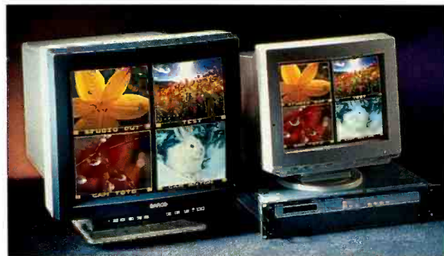
The Barco Vivaldi monitor displays four broadcast-quality NTSC images on a VGA monitor, complete with active titling below the image.
