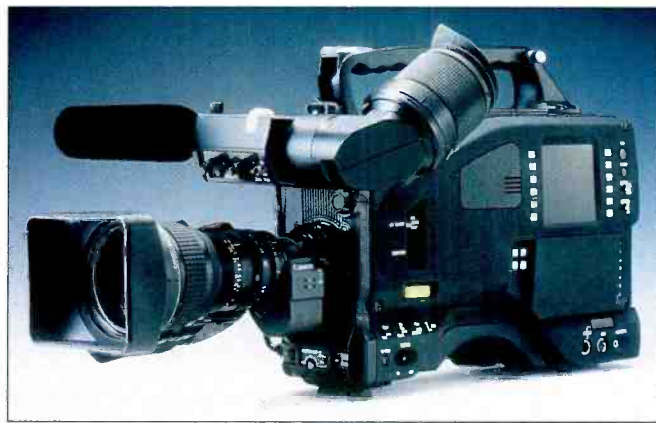
The Avid/Ikegami CamCutter is one of only a few units offering digital disk recording in the field.
