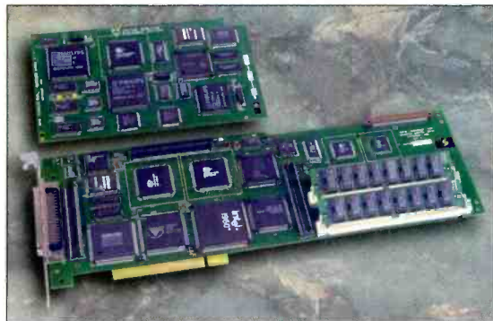
The analog daughtercard and the main board of the Multistream Xpress.
