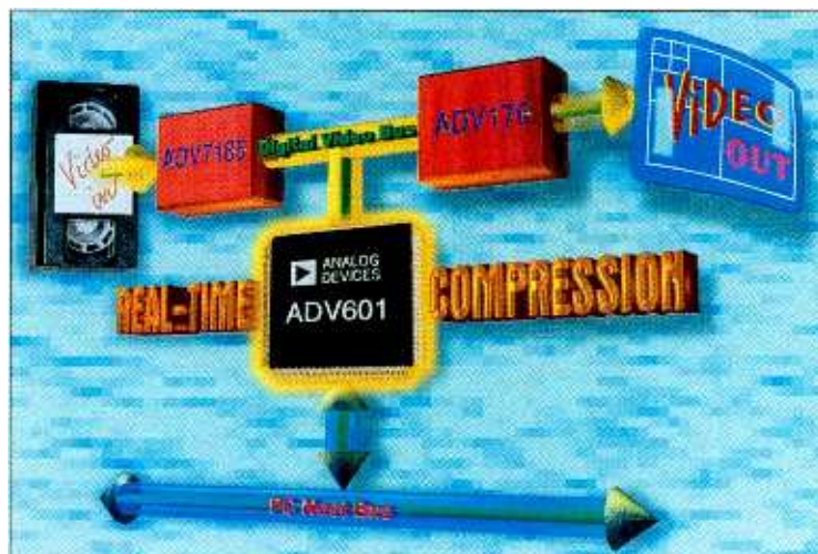
The first wavelet-based IC, Analog Devices' ADV601 provides low cost, high-quality real-time video encoding and playback for PC-based capture and editing.
