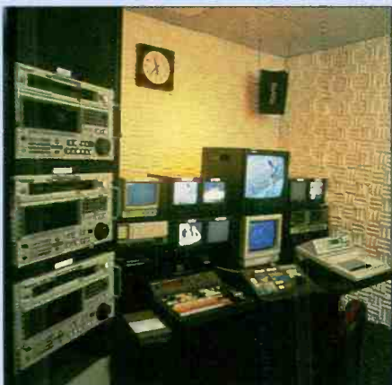
A shot of an AOB edit room, one of seven identical edit rooms. Equipment included three D-3 VTRs and an edit controller.
