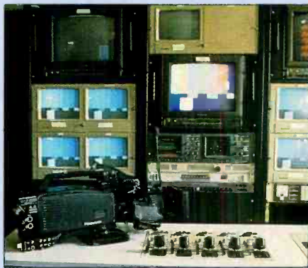
For sports taking place in the Georgia Dome, the AOB used six 60-foot fully equipped trailers. One trailer was devoted to camera control. Shown here is a Panasonic AQ-23W 16:9/4:3 camera and matching control unit. A total of 36 cameras were used inside the Georgia Dome.
