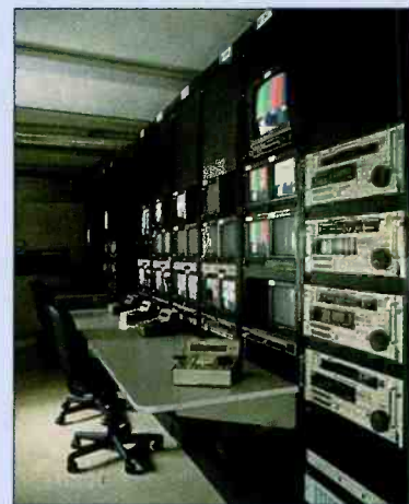
For sports replay at the Georgia Dome, banks of D-3 VTRs and edit controllers were used. The equipment was located in a trailer, just outside the venue.
