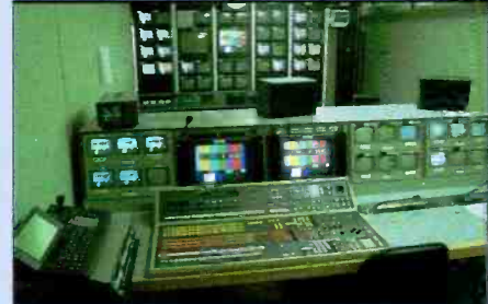
Using production trailers resulted in cost- and space-efficient solutions to editing and control needs. Shown is one control room complete with production switcher and another trailer for distribution.
