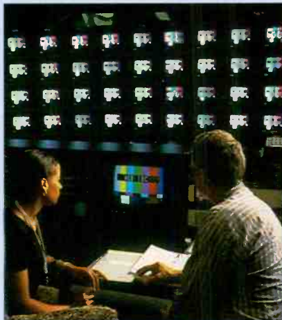
The hub of the Games' broadcast operations center was the International Broadcast Center. The photo shows AOB's transmission center in the IBC. It features a video wall with 72 monitors.
