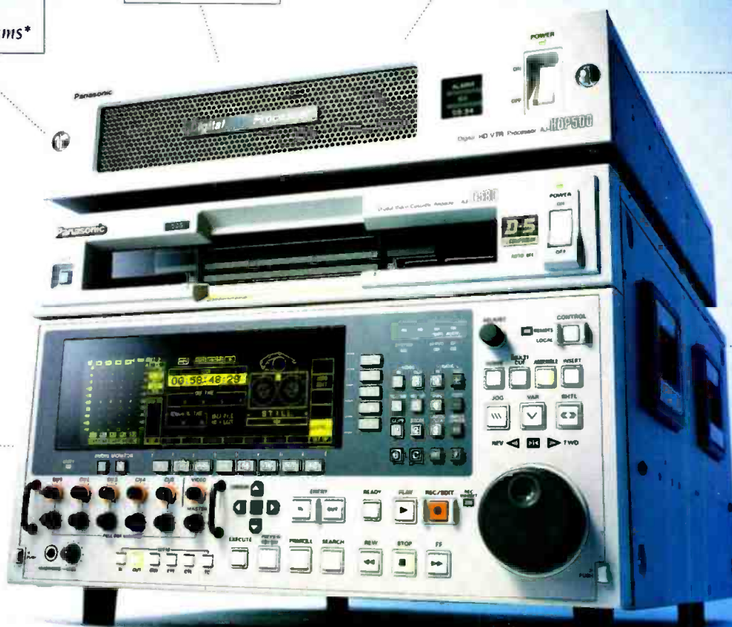
Bottom: AJ-D580 D5 1/2" Component Digital Studio VTR Top: AJ-HDP500 Digital HD VTR Processor
