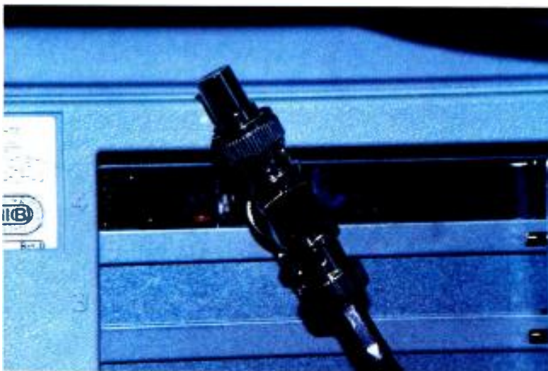
Note the 50Ω terminator connection to one side of the BNC "T."
