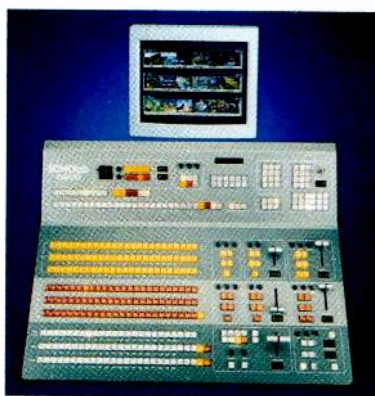
Hidden inside the ECHOlabs 5000's frame is a Pentium computer running Windows NT.
