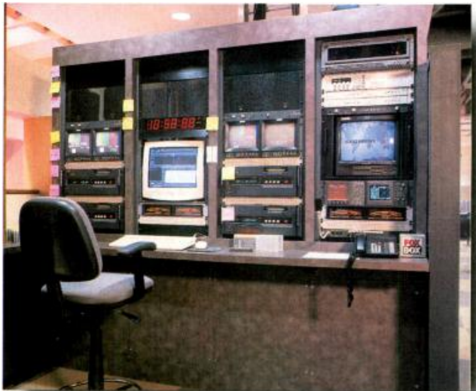
At the news-feed desk, incoming feeds are recorded to tape or directly to shared servers.
