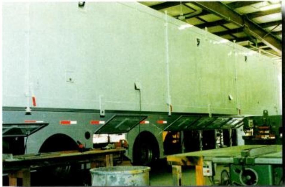
All trucks start out as shells. Here, the NMT HD-1 truck is shown in the Girling Associates factory being modified prior to equipment installation. These modifications included adding "expando" sections, which are needed as much for more people as for equipment.
