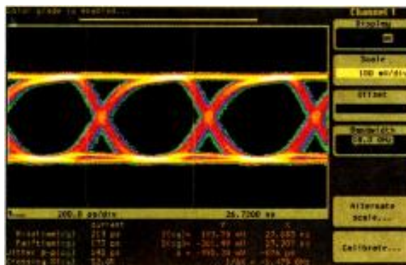
Figure 1. ENVOY 1.5Gbit data output after 75 feet of cable
