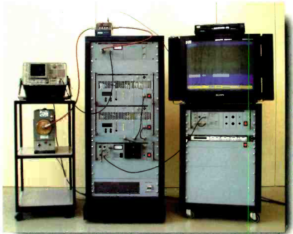
Testing of solid-state ABE Elettronica TX1000/U which employs LD MOS semiconductors. With a digital modulator, units can work with DVB and ATSC signals.
