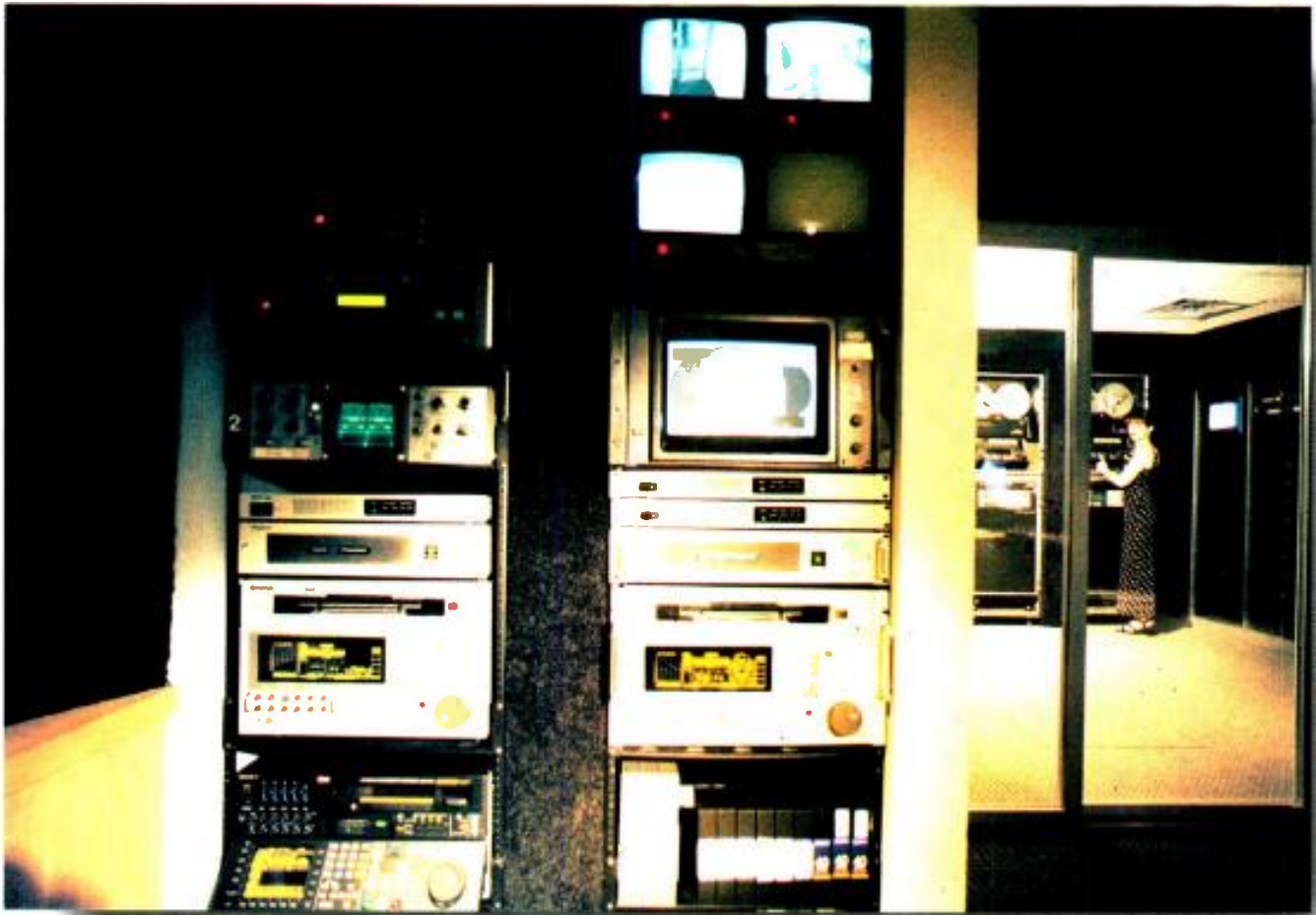
A variety of HD formats are found within HD production facilities, such as COLOSSALVISION in New York, which has HDCAM, D-5 and HD analog one-inch machines.
