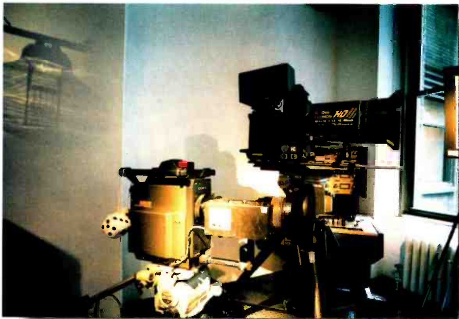
COLOSSALVISION, located in New York, maintains a small museum of older, high-definition equipment. The first commercially available high-definition camera, the Sony HDC-100, can be seen in the foreground. The Ikegami EC-1125, shown in the background, uses three 1¼-inch Plumbicons.
