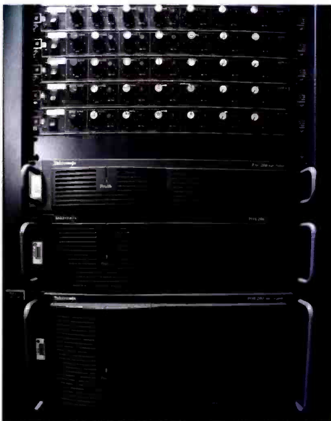
Profile rack showing the PDX208 expansion module, which supports the cuts-only EditStar and the expansion PAC200 audio chassis.
