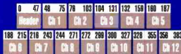
Figure 1: The proposed 384 bit data frames consist of a header followed by 12 28-bit channel packets. Bit numbers are shown above each packet.
