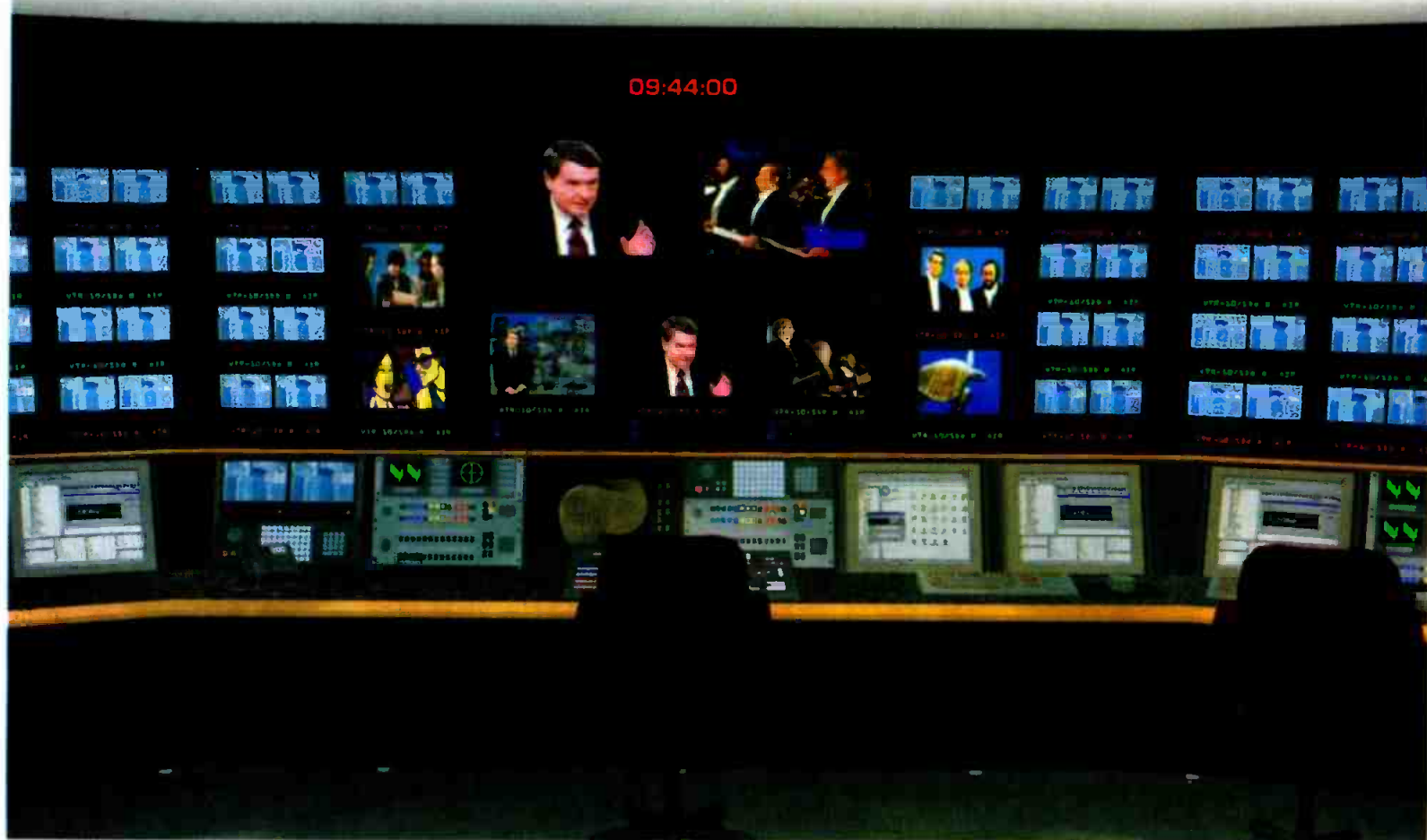
Design concept for multichannel origination control and monitoring station with HD monitoring position.
