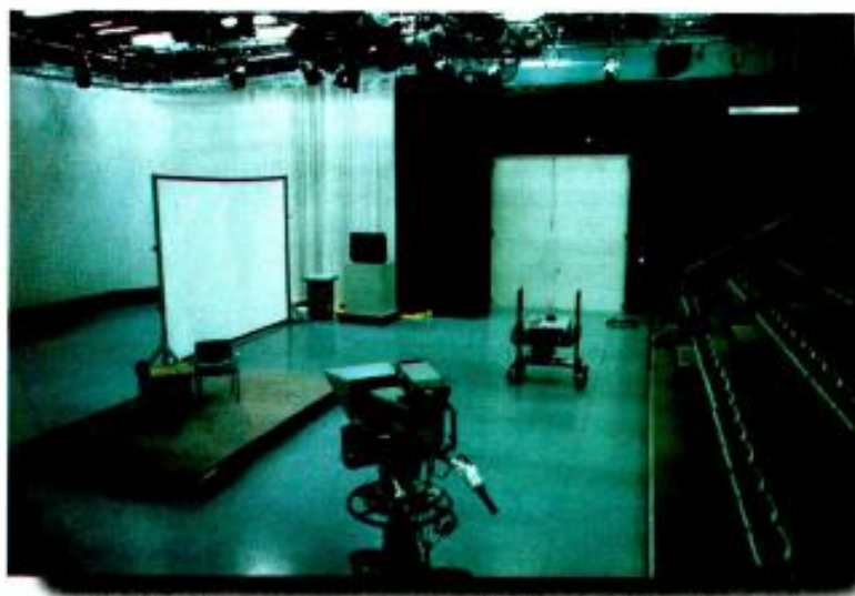
The antenna's view of the studio should be unobstructed. The best placement is usually above camera height, but below the lighting grid.
