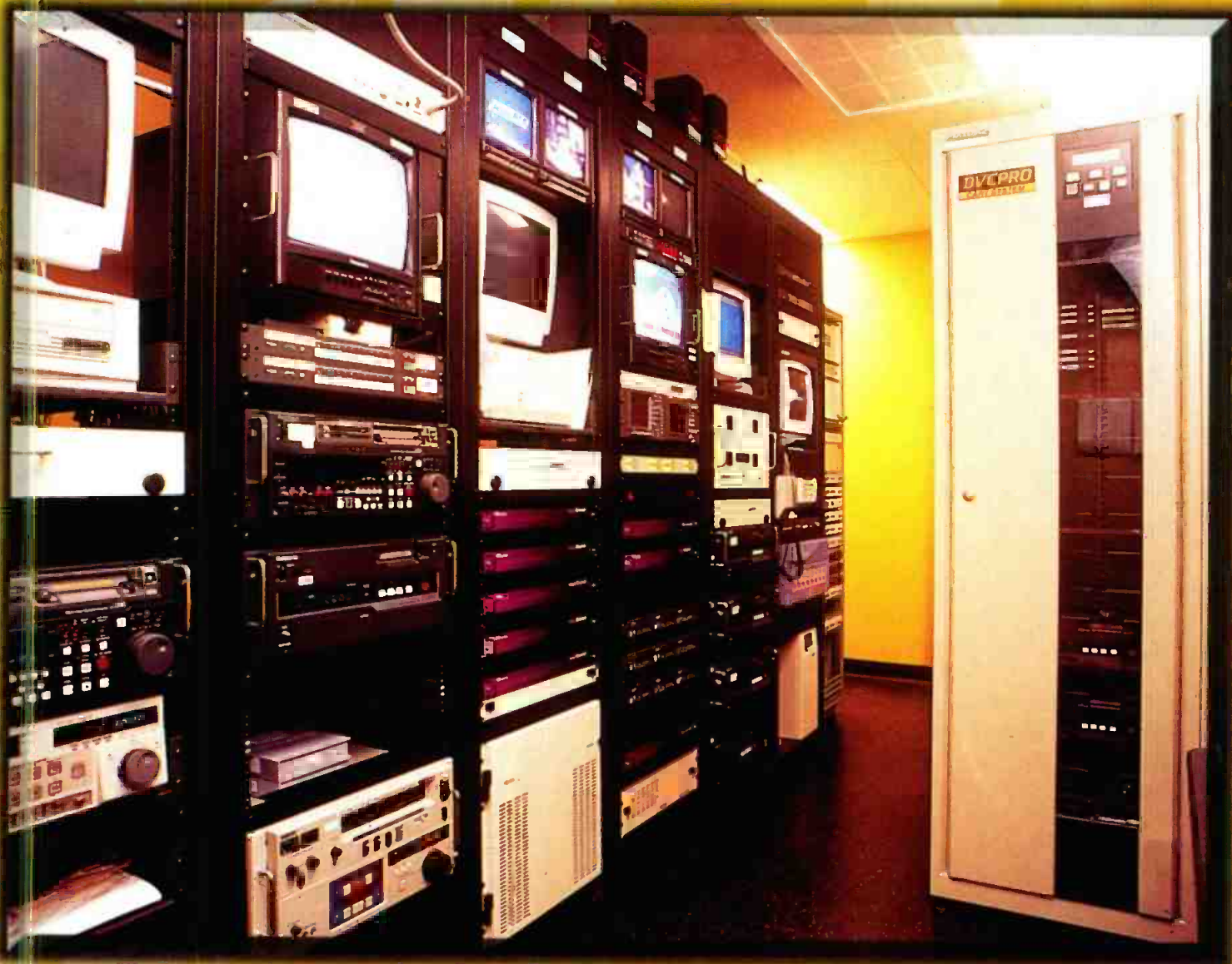
New Orleans Access Television relies on two Panasonic DVCPRO Smart-Cart automated record/playback systems for on-air playback. Shown here is one of the two Smart-Cart systems.
