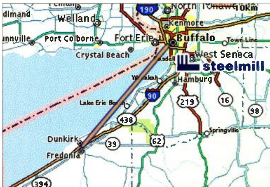
Figure 3: The microwave path that connected the Bills training camp to the studio was close enough to the steel mill to be effected by the radiated steam.
