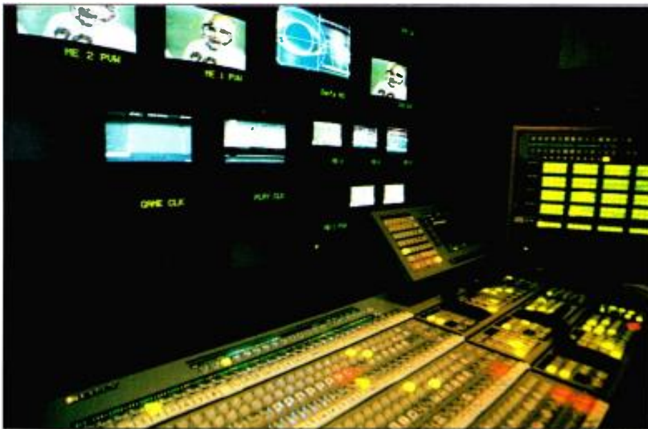
At the heart of NMT's HD-2 truck is the live production area, which includes two Sony HDM-2830 and HDM series high-definition monitors and a HDS-7000 digital switcher with 30 HD digital outputs, three M/E controllers, and a HDME-7000 dual-channel DVE. (Photo credit: Craig Blankenhorn, CBS)
