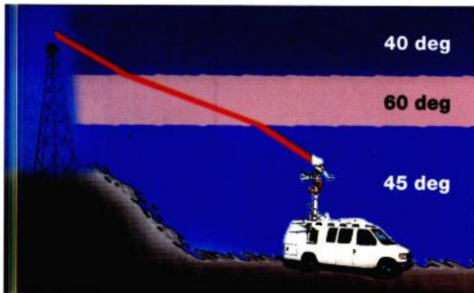
Figure 4: Knowing the height of transmit and receive antennas can help get you around trouble areas.
