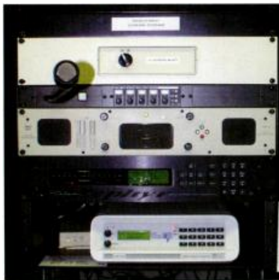
Audio compression technology has enabled the transfer of high quality audio between remotely located studios. Shown here is some of the equipment used to record announcers from remote ISDN-equipped studios and home-based announcers. Equipment includes: Telos Zephyr, APT Reporter, Wohler speakeramp and an RDL Mini Mixer
