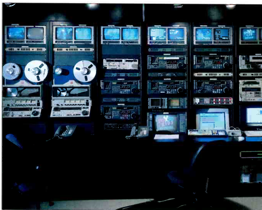
Tape room showing two Sony one-inch machines, JVC Digital S tape machines and a Panasonic M-2 tape machine.
