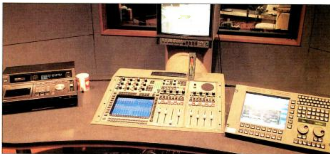
Henninger Digital Audio's Capitol Facility is equipped with AMS Neve' Logic 3 post-production systems and Audiofile DAWs.
