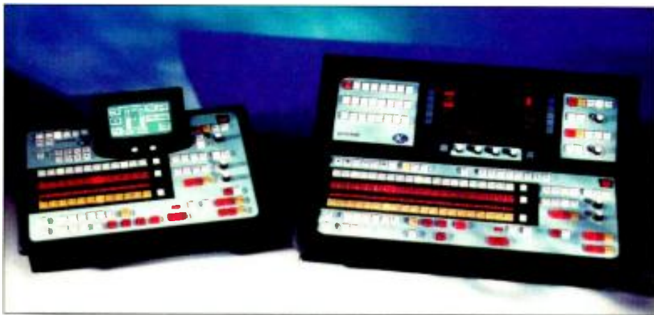
Pro-Bel automated master control goes beyond a serial link with rudimentary controls by offering built-in automation buttons in the master control, video HUD of schedule and under-monitor displays in the master control monitor walls, among other features.
