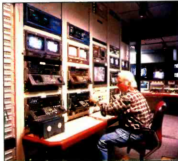
NBC engineer Marv Richardson works with Sony HDW-500 HDCAM VTRs in "The Tonight Show" edit tape area. The show is the first network offering to adopt an HD format. Photo by Concept: Benson & Rice. Courtesy of Sony.
