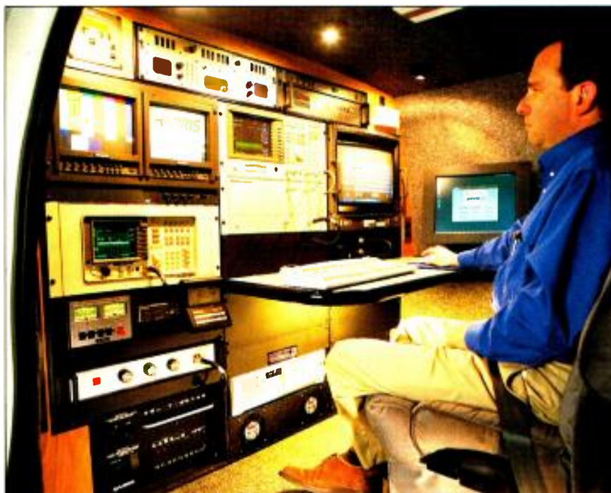
A Harris operator sits comfortably inside the van collecting data during the field test. The keyboard provides easy input of information to the computer program controlling the HP 89441V vector signal analyzer.
