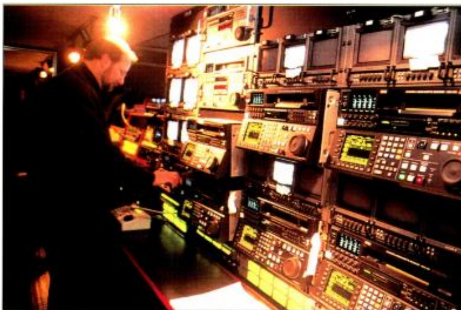
Currently one of the few formats available for HD acquisition and production, these HDCAM VTRs were used by KTVU for the Chinese New Year parade.
