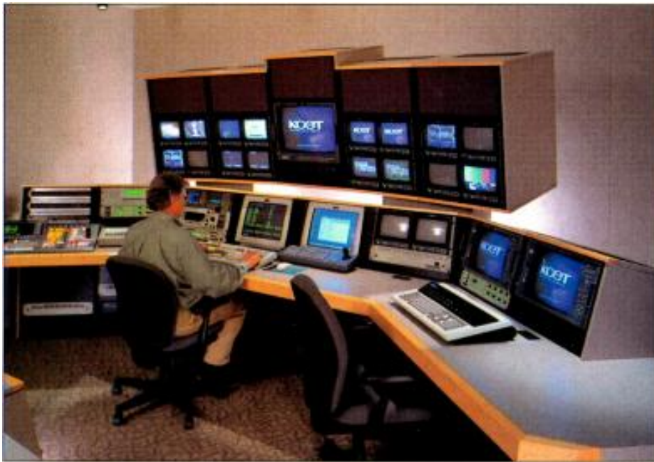
Each all-digital edit room is equipped with an Editware nonlinear driver to control multiple channels of Tektronix Profile and Sony SX tape. Photo by Sandra Williams.
