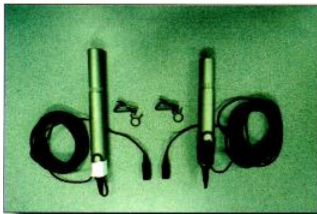
Typical lavalier mics have small capsules (elements) that are connected to the remainder of the electronics using a thin wire. Small clips allow the elements to be attached. Some units are sealed against moisture and can even be spray painted.
