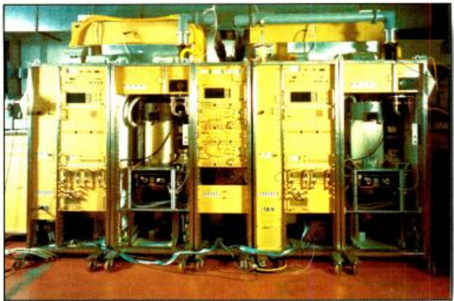
An Iteco 604K 80kW IOT undergoing final acceptance tests at the factory.
