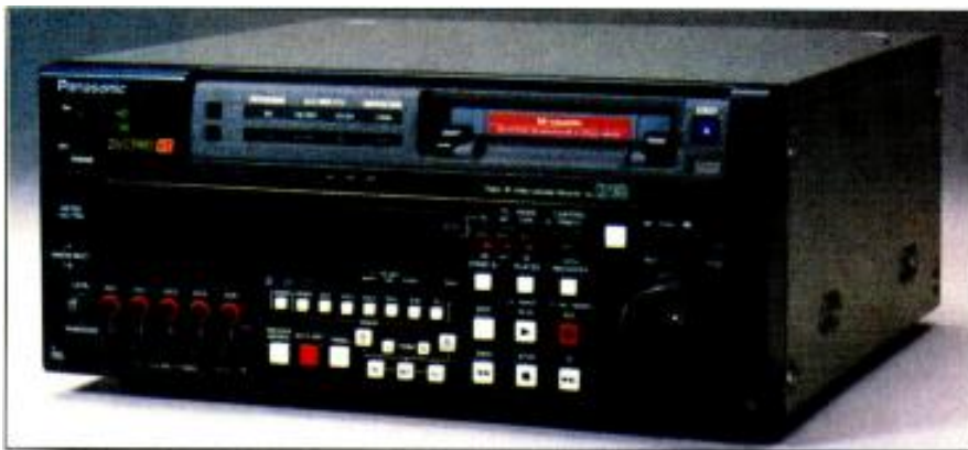
Panasonic's AJ-HD150 DVCPRO-HD VTR can playback both DVCPRO and DVCPRO 50 recorded tapes.
