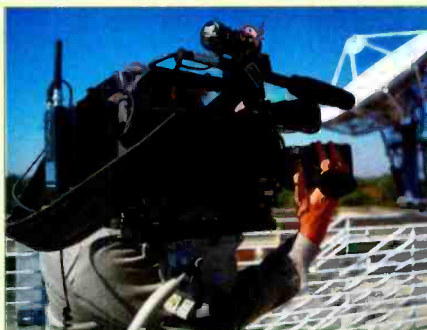
A good shooter is prepared for any situation. The setup above features a wireless receiver, shotgun mic, camera-mounted light and fluid-filled camera head on tripod.
