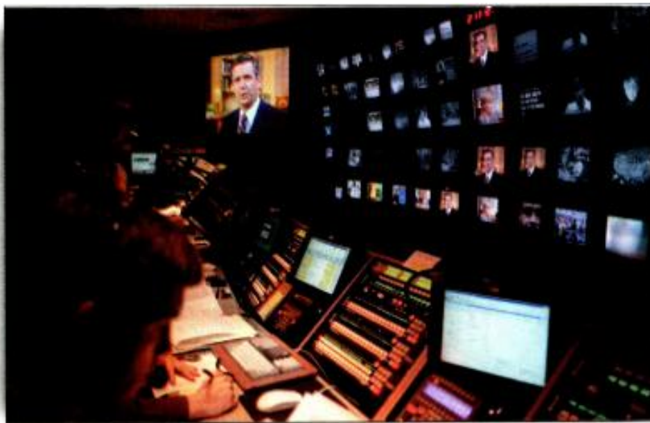
Production staff in GMA 's state-of-the-art control room. Over a dozen PC stations, called pods, are situated throughout the production control room and other technical areas. The PCs themselves are located together in the central equipment room. (Photo courtesy of Ida Mae Astute/ABC)
