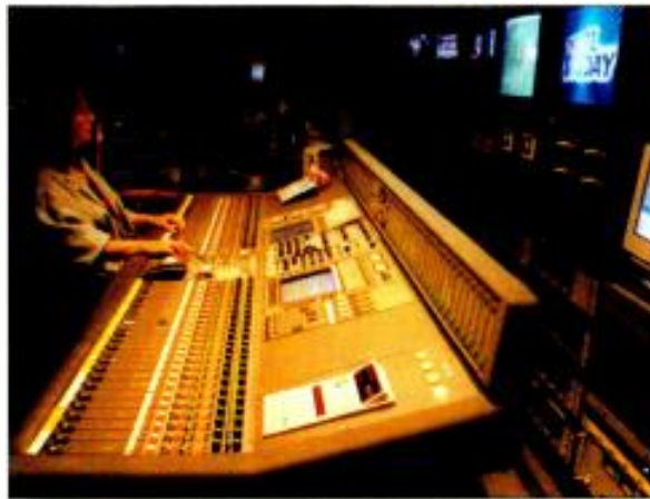
Digital consoles, such as this AMS Neve Libra Live broadcast production console at CBS's control room #43 at its New York headquarters, must be matched to a facility's needs and budget.
