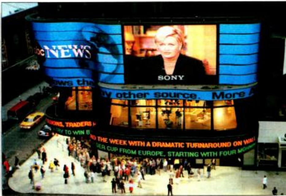
The 855-square-foot Marquee features the Sony JTS-L15 LED display, the largest JumboTron in the U.S. used as an outdoor billboard. (Photo courtesy of Ida Mae Astute/ABC)
