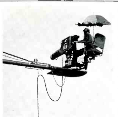
Six versatile camera cranes, previously used in filming classics like "Cleopatra," were used in televising the second annual "CBS Golf Classic." Camera booms on the self-propelled vehicles stay level, even on hillside positions. Cranes and cameras are battery-powered for "silent" operation. The entire event of 14 elimination matches, each 18-holes, was recorded on Scotch video tape and later televised on Saturday afternoons over CBS network.
