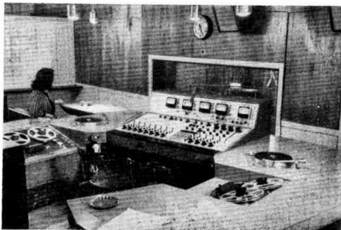
Hardman Associates main control console is custom-built for mixing tape, disc, and mic inputs in multiple units.
