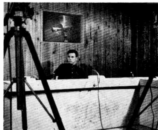
Local origination studio viewed from camera position in Studio B. Directly behind newscaster is frosted glass rear-projection screen lit up with a slide projected from the engineering booth. Knotty cedar paneling fits into decor.
