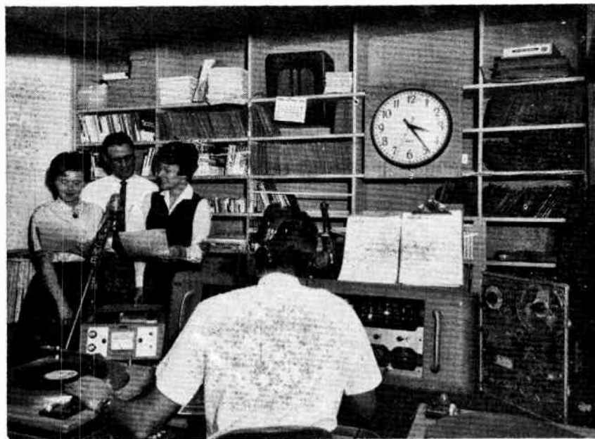
WCME recording studio has a Gates console, Ampex 601 and 350, and older Magnecord (used mostly for editing), and a Tapecaster cartridge machine for dubbing. In production session shown here are (l-r) Mrs. Roma Gibbs, William McKeen, gen. & sales mgr.; Mrs. Pat Vickers (British secretary), and Jim Roberts, director of operations.
