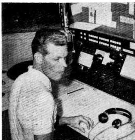
WFUN control room console has remote control pushbuttons for MacKenzie tape decks, 3 cartridge tape playbacks, echo, filter, time tone, etc., a total of 55 illuminated buttons. All amplifiers—completely solid-state—have been removed from console and studio to eliminate the necessity of disturbing the announcer for maintenance. Standby power is supplied by a transistorized inverter with automatic transfer.
