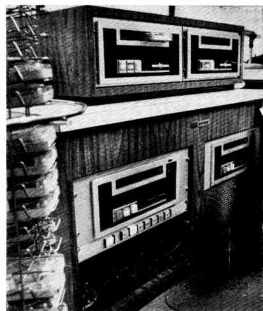
WABC main air studio facilities include 6 remote control ATC cartridge playbacks (two are on opposite side of console desk), a turntable, echo chamber, and Ampex reel-to-reel recorders.
