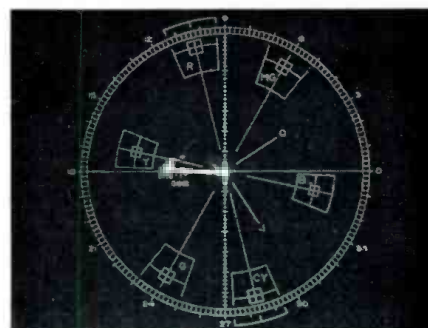
Fig. 2. Display of a distorted modulated staircase, viewed on the Vectorscope. Phase is displayed on the graticule in a circular direction and amplitude in terms of distance from the center.
