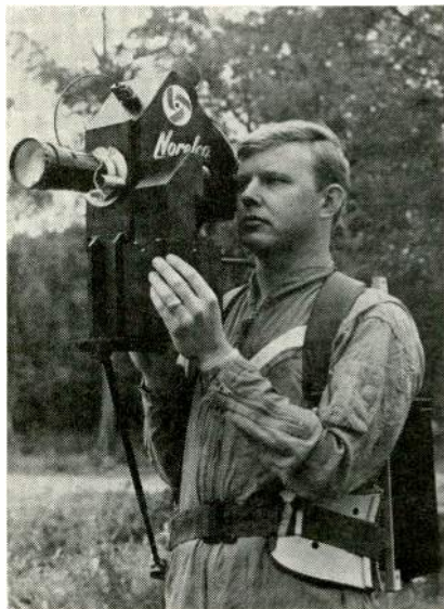
Left. Prototype version of the 44-pound Norelco PCP-70 portable color camera which produces broadcast quality signals equivalent to that of the PC-70.
