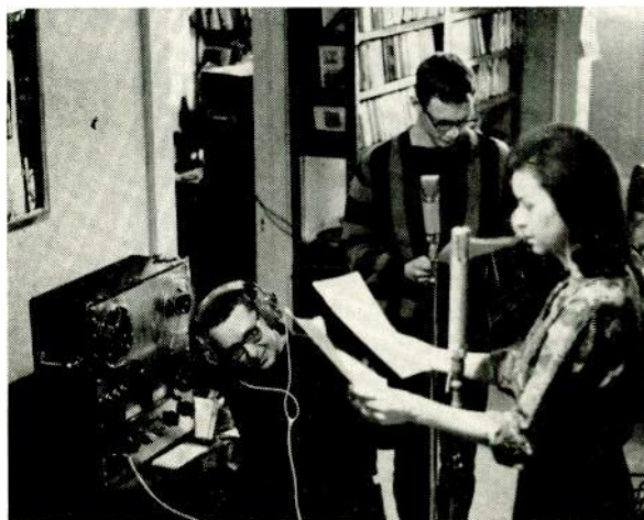
Above The author (1) adjusts an AKG C-12 mic for the actress. Actor is using a Synchron Au7a mic. Patterns are perpendicular.
