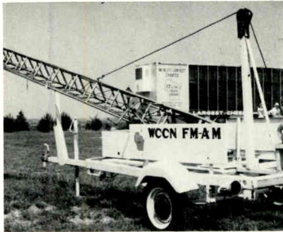
Trailer-mounted crank-up antenna facilitates remote operation. Last 20-ft section isn't extended till distance from antenna shown on p. 63 exceeds 25 miles.
