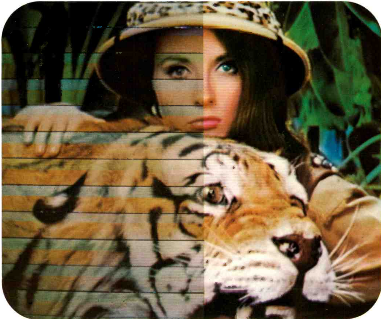
Unretouched photographs of 21" studio monitor. Photographic data: Rolleiflex C-3, CPS color negative film — ASA 100, 1/15 second at f/5.6
