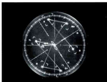
Type 520 Vector Display of VITS color bars conforms to EIA Spec. RS189. Signal Source — Type 140 NTSC Test Signal Generator.
