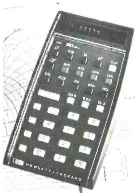
Fig. 2 A close-up of the HP-35 pocket calculator shows the possible functions which will give a readout on the LED's.
