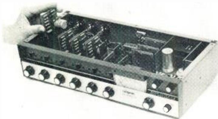
In Langevin's AMIA mixer, two continuous equalizer controls allow adjustment of high and low frequencies.
