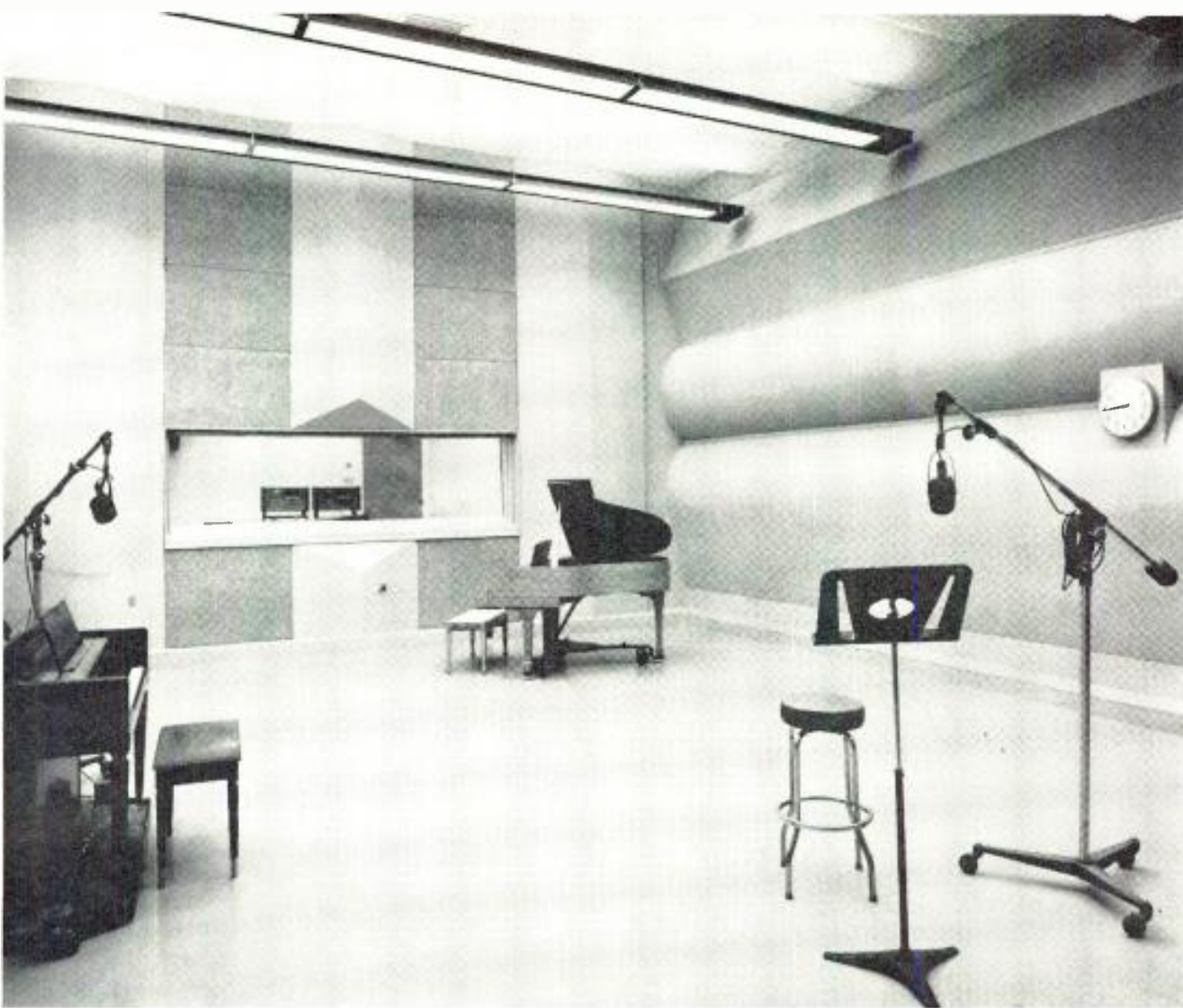
A rarity outside of network centers, this 30 by 40 studio with acoustically curved walls and ceiling is used for radio.
