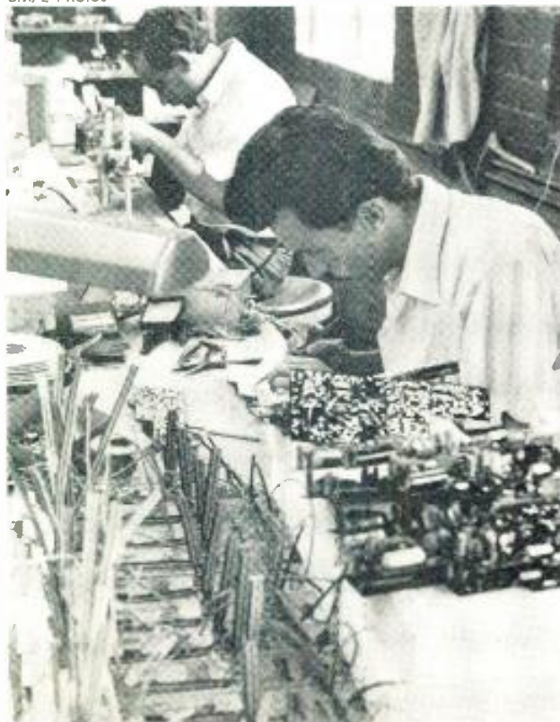
Production-line inspector touches up dip-soldered circuit board with pencil soldering iron.
