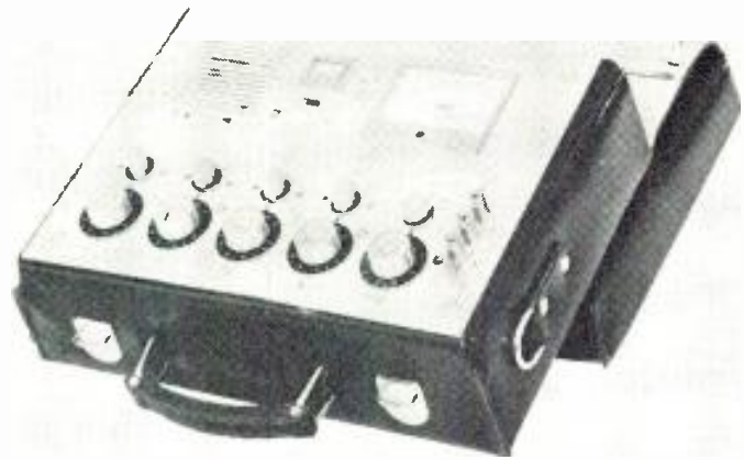
Line output of EMT 104 appears on panel binding posts to accept bare felco wires if necessary.
