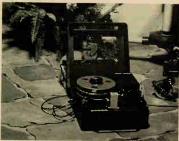
New Bosch BCN 20 hand-held VTR which can be used for field production recording.
