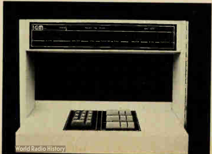
New fixed-cart system, the Carostat (above), was introduced by SMC at Las Vegas. It has 12 or 24 carts, each with own playback system. The cart cued in moves 1/16th inch to drive system.
