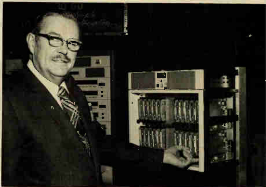
New fixed-cart system, the Carostat (above), was introduced by SMC at Las Vegas. It has 12 or 24 carts, each with own playback system. The cart cued in moves 1/16th inch to drive system.
