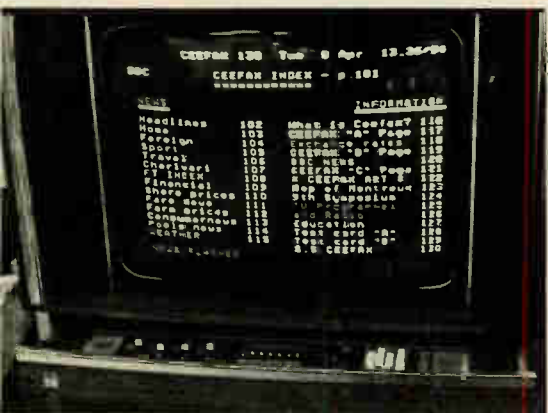
TV set modified with decoder to pick up data transmitted during horizontal blanking. Numbers are different "pages" viewer can select.
