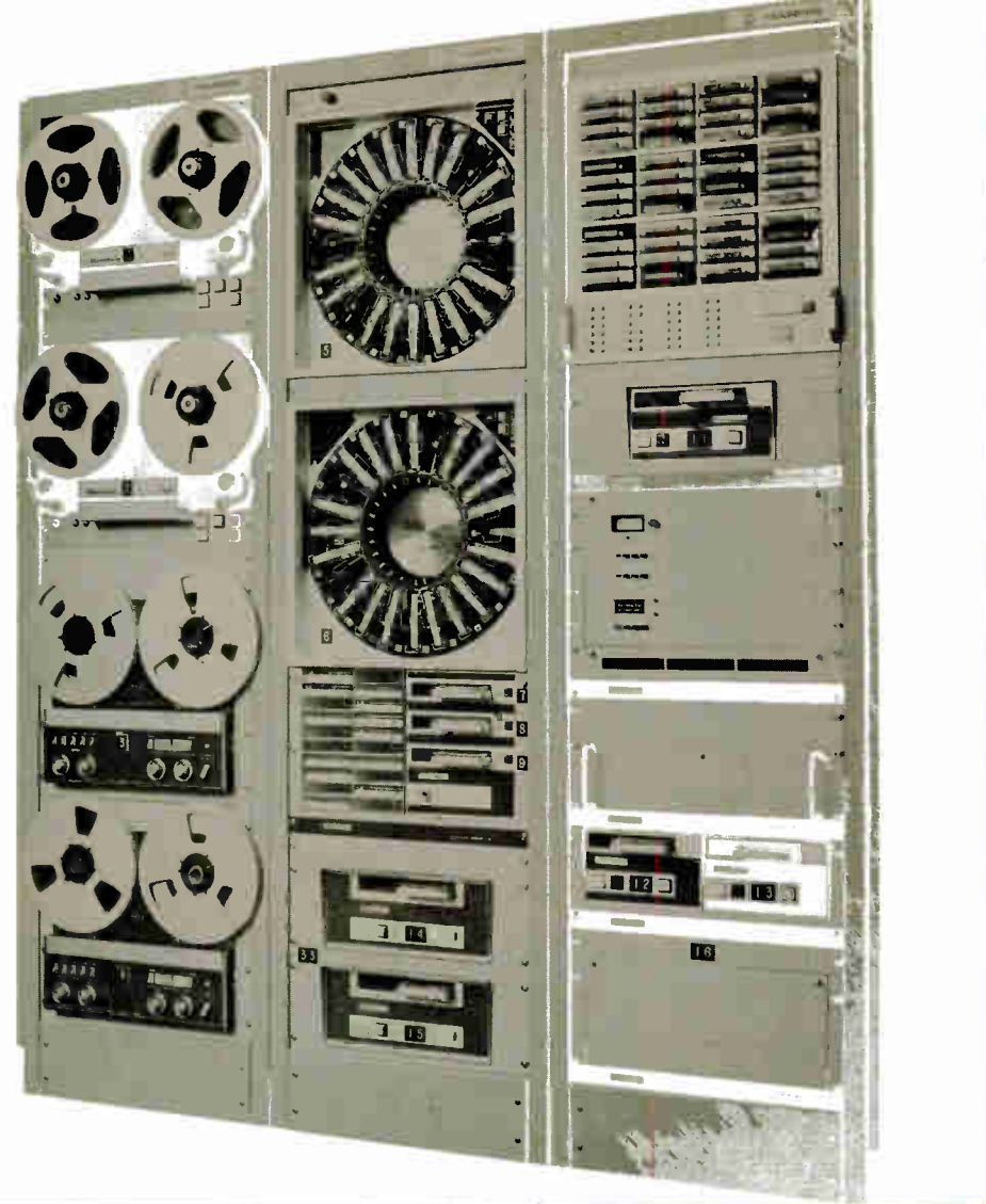
Harris System 90 (left) has minicomputer, memory, audio switching and power supply in third rack, below multicart machine. Example shown has one audiofile, two Carousels, four reel-to-reel machines; other configurations are readily made (system handles up to 16 inputs).
