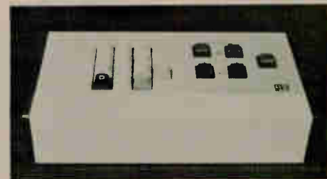
Control box for Audio Services' System 1 automation system (above) can be used remote from studio, connected to studio by FSK digital signals over telephone lines. Remote man has same control of system as in studio.
