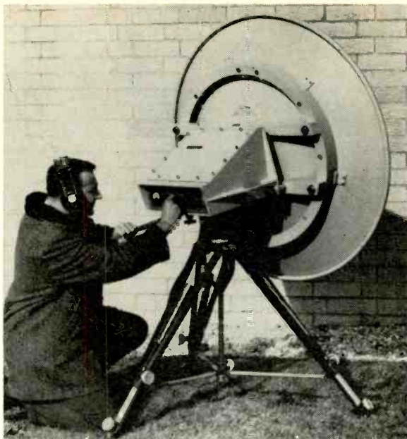
MRS-AP series of microwave links from RHG Electronics Laboratory has output power from 0.25 to 4 watts.
