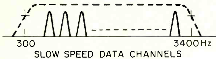
Fig. 2. Slow-speed data channels (facsimile, meter reading, computer data) can be accommodated in the same spectrum space that serves telephone communications.
