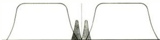
Fig. 2. Typical AM frequency spectrum showing carrier (center), PM*PM signals (dark areas) and AM sidebands (light areas).
