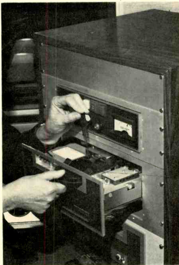
Adjustable guide on the Marathon cartridge is located for easy access during operation.
