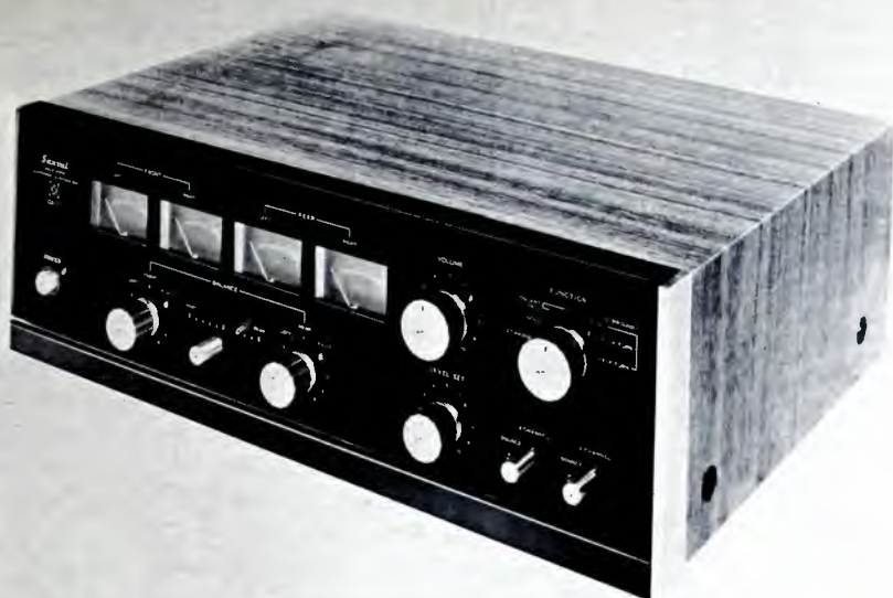
This decoder from Sansui can create four-channel sound from conventional stereo records as well as decode E-V or Sansui encoded records.
