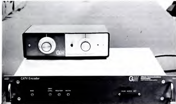
Simplicity is feature of Athena system. Encoder is located at headend. Decoder is a modified Gamut 26 converter.
