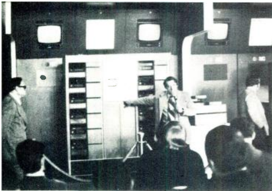
IVC's automatic cartridge player, the BCR-200, uses a helical format.
