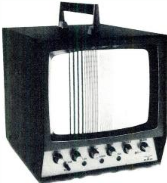
Fig. 3A. Multiburst test signal gives quick check on system's high frequency response. Photo courtesy Ultra Audio Products.
