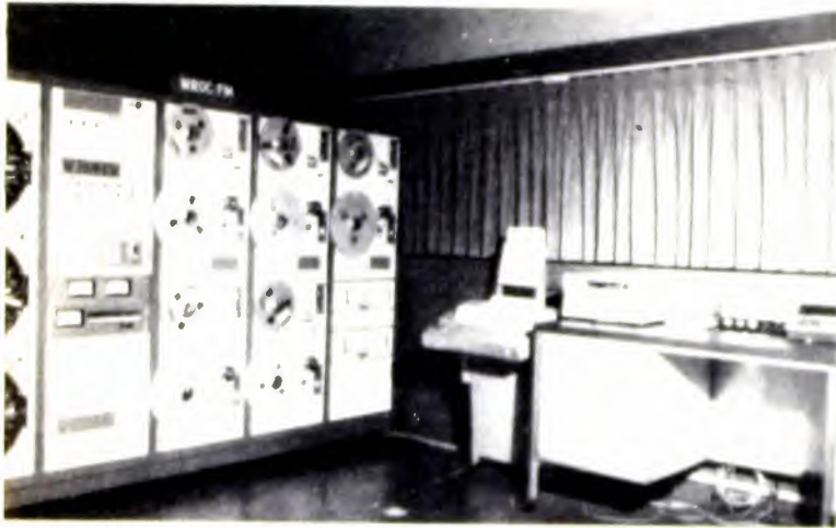
Sono-Mag DP-1 at WROC, Rochester, has five Scully tape decks (right hand bays), three Carousels (left, left end), with control equipment in center including full random access, and storage of 2048 events.
