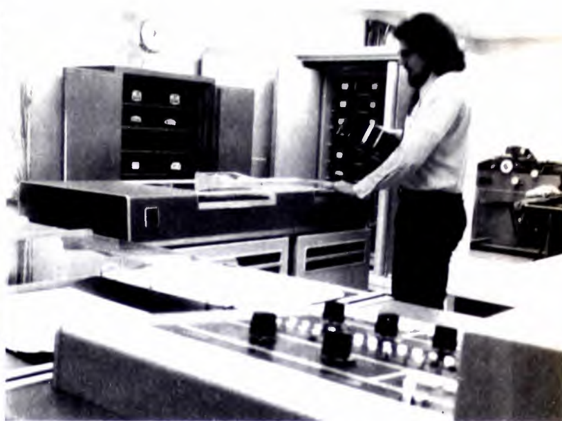
Numbers and artists of each selection are entered on magnetic disc storage in computer, for selection process which maximizes desired format and voids quick repeats of artists.
