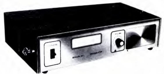
"BTVision" decoder has roll of strip tickets inside with complete record of programs watched. The roll is collected monthly for billing.
