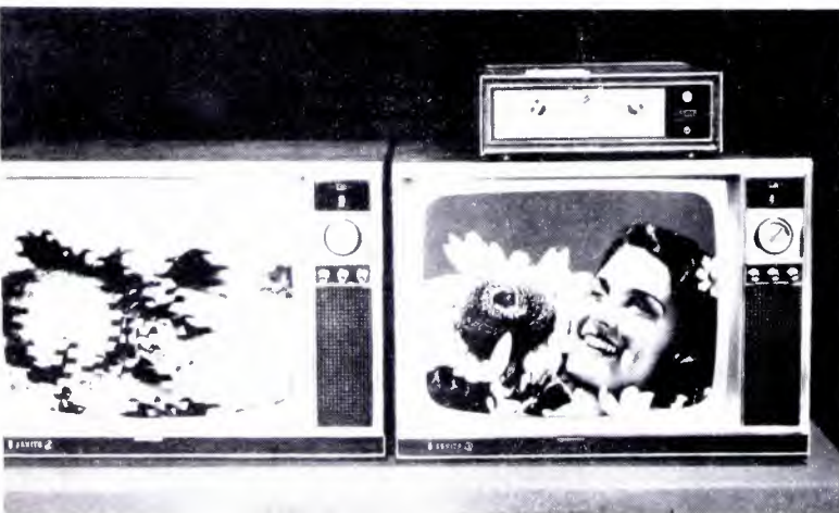
"Phonevision," Zenith's pay-TV system, produces scrambled picture (like that on left set above) if no decoding is available. With decoder (top of right set) the picture is restored to full visibility.
