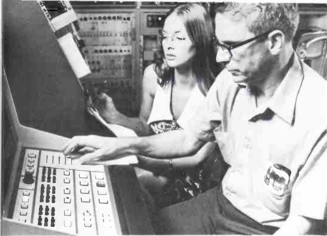
Automated and semi-automated videotape editing is becoming standard in the tape production houses (and in larger broadcast stations as well). Here Bruce Harris of WFAA Productions, Dallas, assembles a videotape program with the help of the Ampex RA-4000 random-access timecode editor.
