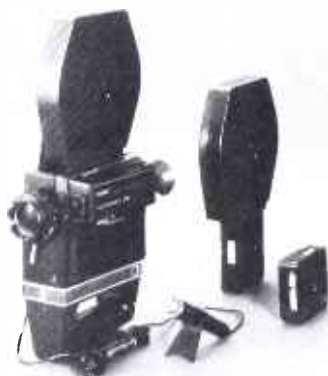
Magnavox Chromavue 440 is one of the portable video cameras newly on the market which are getting tryouts for some areas of television news gathering. Others are listed in box on earlier page. Such portables will ordinarily involve a backpack with the electronics for the cameraman, plus a VTR carried by a second man or in accompanying mobile unit.
