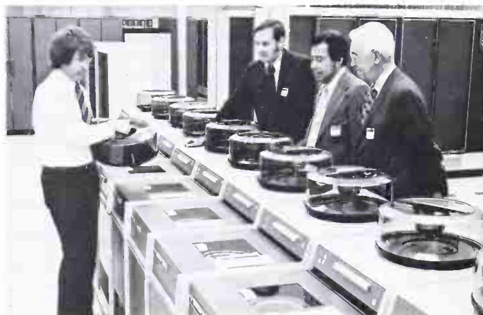
Mass data storage at headquarters of Compu/Net system is on magnetic discs. Each pack (ten discs) can hold over 110 million characters.
