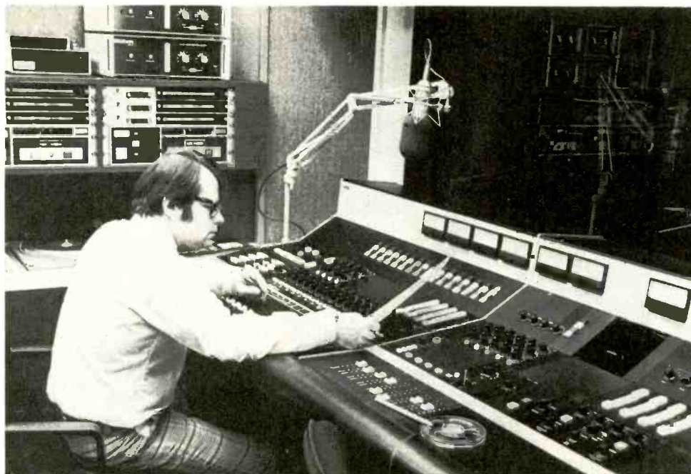
Control console for Production Room #1 is a full 16-input, 4-output board capable of quad, stereo, mono mixing.
