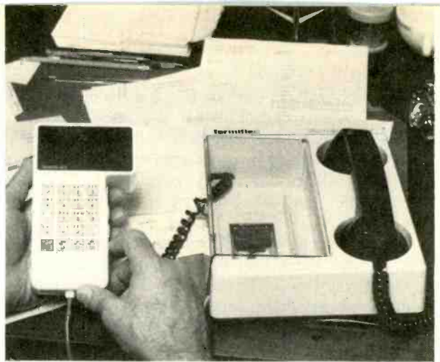
New Termiflex brief-case terminal permits a salesman on the road to query the station's computer.
