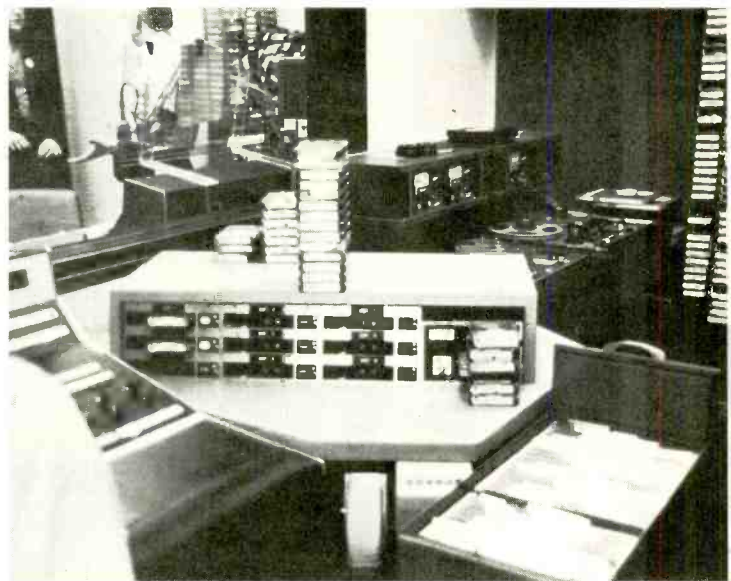
The bank of nine ITC cart machines serve as the program source for most of the regular programming. Carts can be set up for automatic sequencing in any order; sequence can be held, restarted, dumped by operator.
