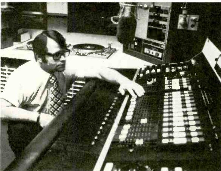
Author Klabunde sits in front of control console. This unit is actually in Production Room #2 but is exact duplicate of master control console, and can take over the master control function if necessary. Buttons used by DJ to control automation functions are on panel at far end of console (see story).
