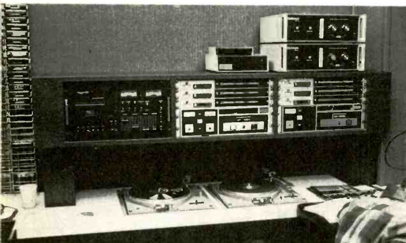
Production studio equipment includes turntables and cart machines, equalizers, Dolby noise reduction units, reverb, Nakamichi cassette machine, Multisync.
