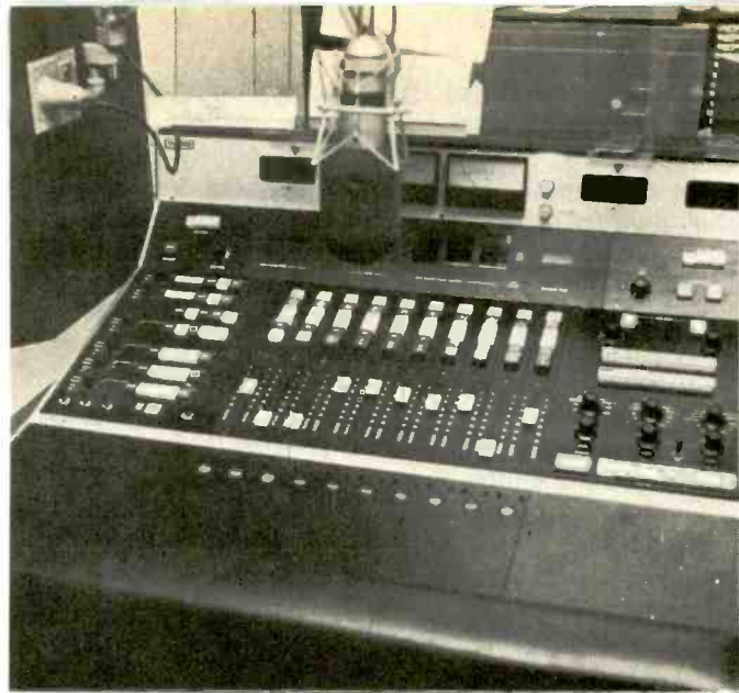
Console in news control room is tied in with automatic time gates that set up sequence of non-music programming for as long as a week in advance.
