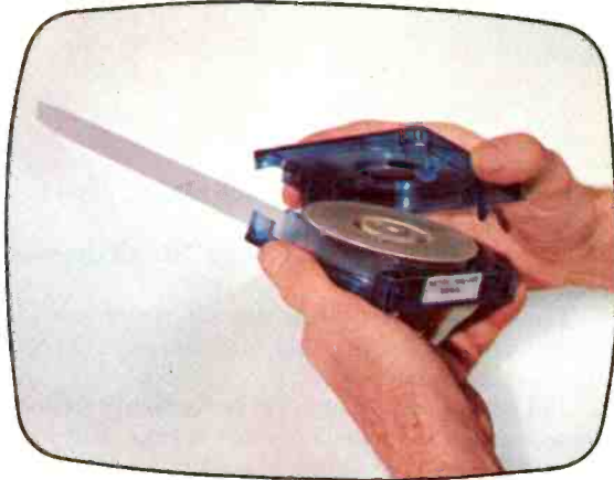
A special Mylar leader is spliced onto each film segment. Film is inserted into a cartridge—no further film handling.
