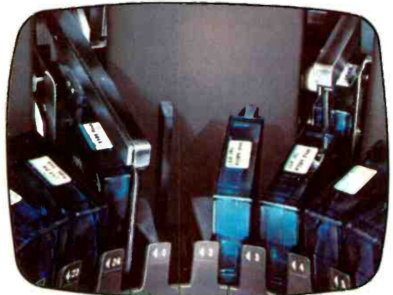
As the first reel rewinds and is replaced in the magazine, the second projector runs film from the next cartridge.
