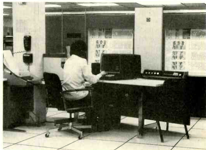
Programmer sitting at control panel of B6700 computer which handles both radio and TV stations.
