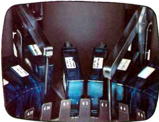
A cartridge is drawn into the machine on cue, shown by one of the two projectors, then rewound, all automatically.
