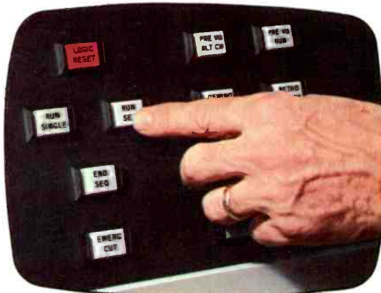
The TCP-1624 will play one cartridge and stop, or will play cartridges continuously until it receives an order to stop.
