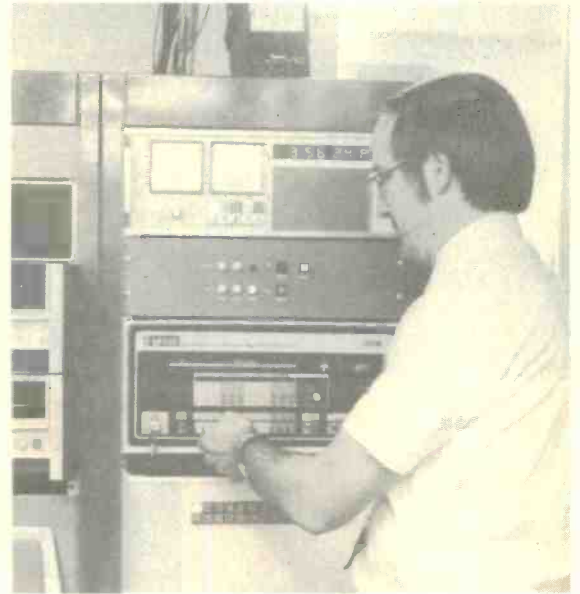
The 770 includes the PDP-8 computer which has a 20K computer word memory. One disc adds another 1600K. Pictured is Dir. of Tech Ops Larry Conti.
