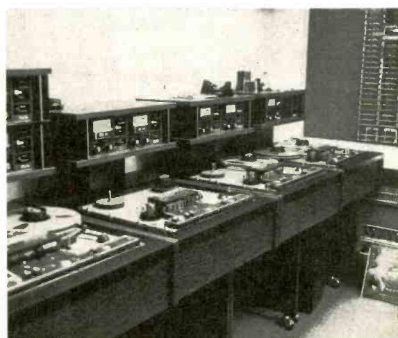
Bank of Scully tape machines in Production Room #1 includes models for 4-track, 2-track and mono recording.
