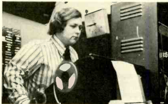
John Preuter, production manager, puts the 25 Hz cue tone on a commercial which will alert announcer for "live" talk.
