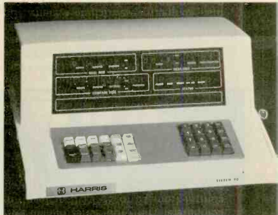
Control console for Harris System 90 (below) can be remote from main racks; two or more consoles can be used. System is fully operated from keyboard; displays include real time, "compare" (or running) time, current event, next event, edit operation, system status.
