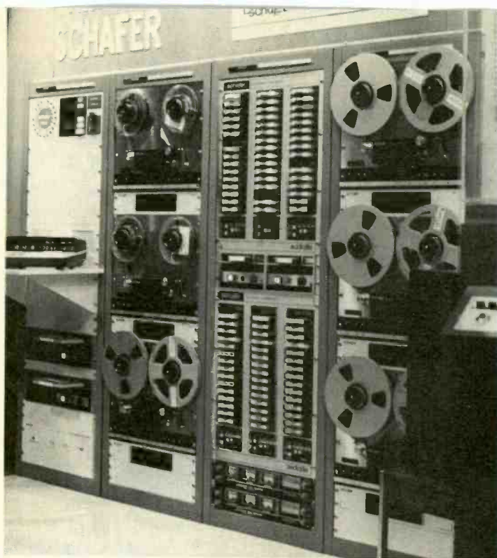
Schafer 903 system (above) with MOS memory is shown with two Audiofiles (third rack), six reel-to-reel machines, complete control electronics (first rack).
