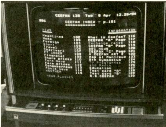
TV set modified with decoder to pick up data transmitted during horizontal blanking. Numbers are different "pages" viewer can select.
