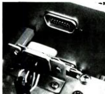
All leads to the deck go through this plug-in connector.
