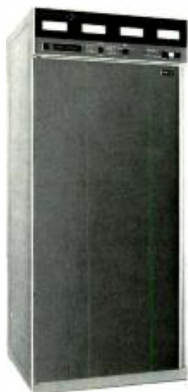
MW-1A, 100% solid-state one kilowatt transmitter
