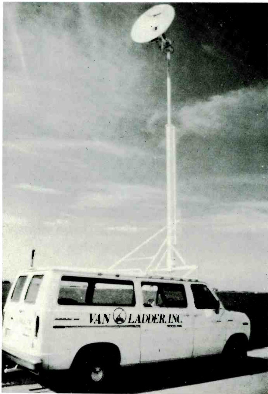
Microwave will be hot at NAB with a lot of new equipment. Here, a Van Ladder 29 ft. telescoping boom is shown.
