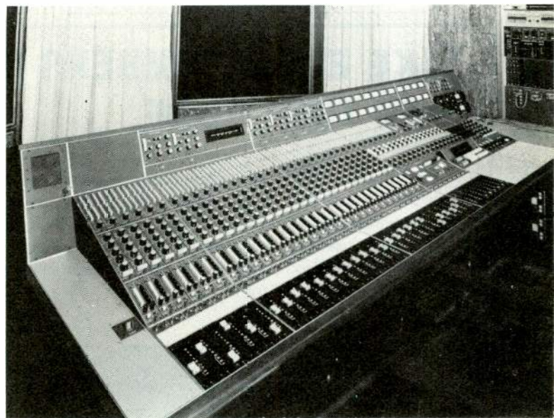
Neve "Computer Assisted" mix-down system includes control panel and readout installed in right end of console; faders are operated by servos, with manual override.
