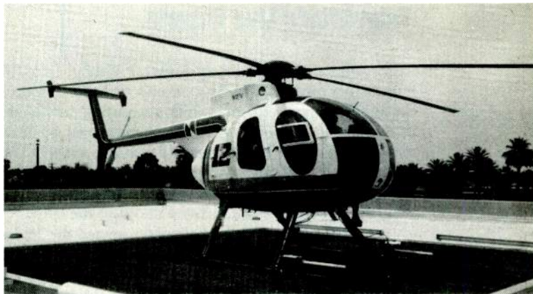
KPNX, Phoenix, uses its Tayburn-designed helicopter microwave system as both a repeater and a camera platform on Memorial Day to cover activities on a lake
