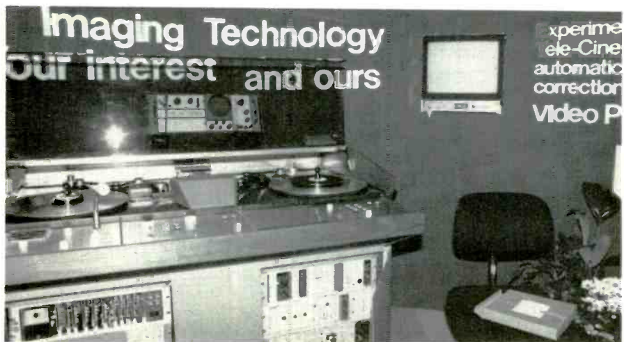
Eastman Kodak showed a new telecine (below) especially designed for high speed news film. Resolution lost due to pushing is restored in this new unit
